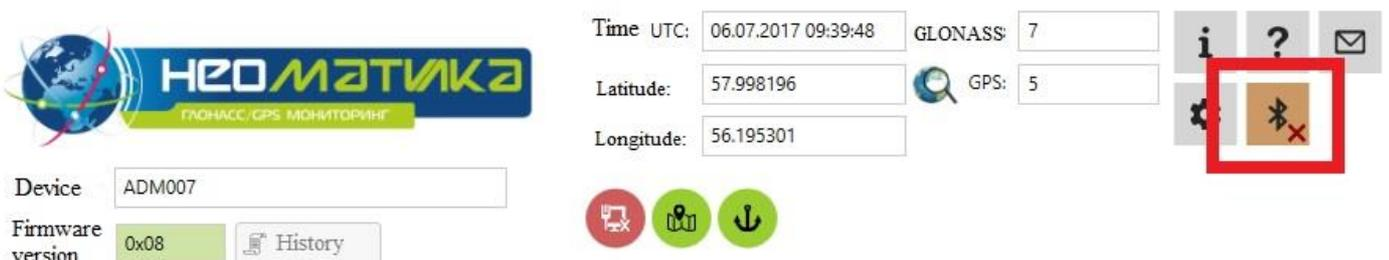
Figure 6 – ADM Configurator: the "disable device" button
